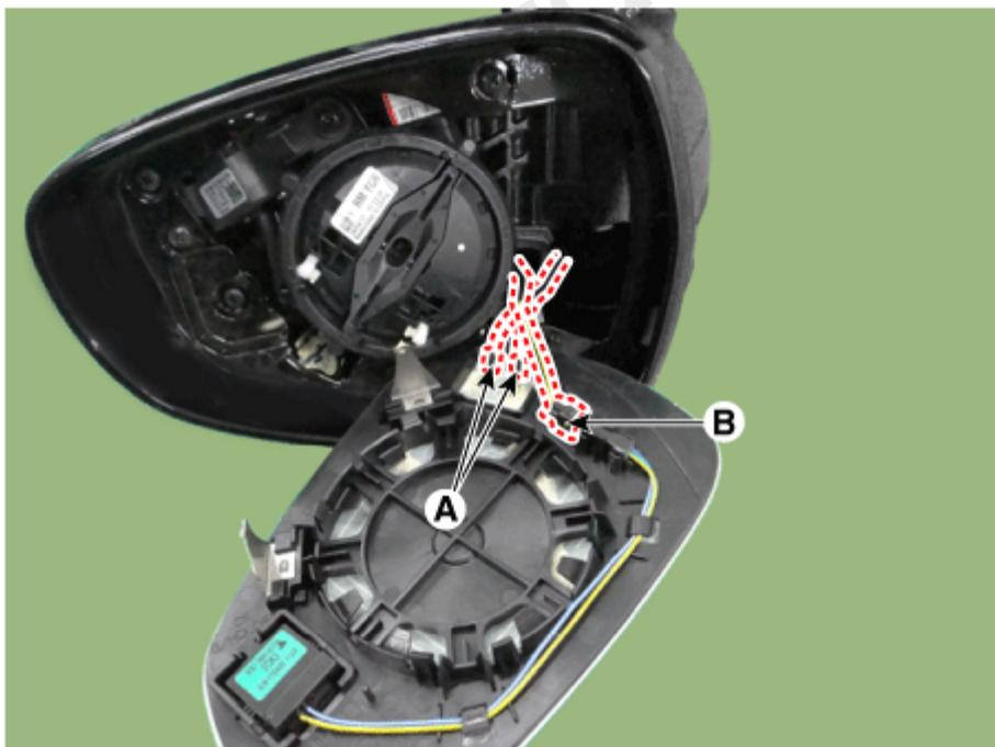
4. Remove the housing cover mounting screw.
